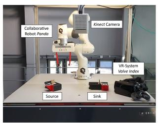
Figure 7.: Setup of the experimental environment with the collaborative robot Panda, the depth camera Azure Kinect, and the teleoperation system with the Valve Index VR glasses
