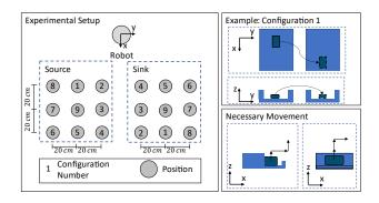
Figure 10.: Setup for the second experimental series to compare the presented approach with unsegmented DMPs performing the described task with start position in source and goal position in sink for each configuration number.
