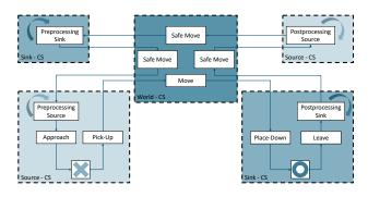
Figure 5.: Conceptual description of the 5+5 Steps of the Material Handling Loop with trajectory segments (white boxes), the grasp (x) and the release (o) point and the reference coordinate systems (CS) source, sink and world, relative to whom the trajectories are executed.
