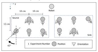
Figure 9.: Experimental setup for evaluating the adaptability of the approach by spreading source and sink positions and rotating them.
