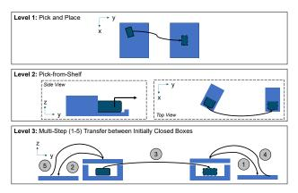
Figure 8.: Scenarios to be evaluated with various levels of difficulty to represent various logistics tasks.
