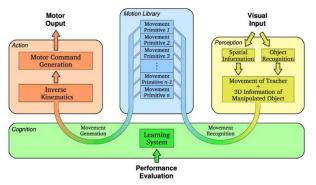
Figure 4.: Schematic representation of the DMP-based control of a movement using a library of movement primitives [8].
