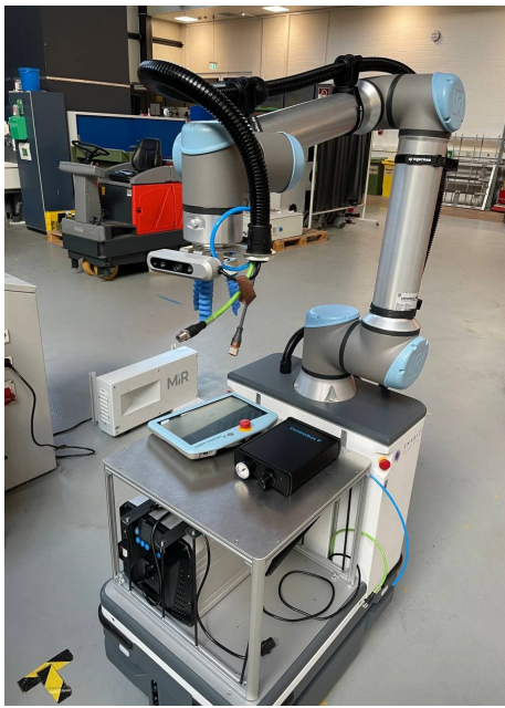
Figure 8. The robotic Arm and Softgripper system
