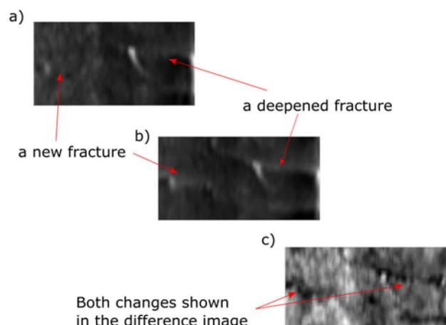
Figure 6. Training data: a) surface of a fracture from measurement 1; b) surface of the same fracture from a subsequent measurement 2 (one month later); c) difference between the two measurements
