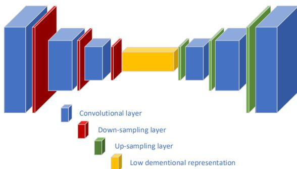
Figure 5. Structure of proposed convolutional autoencoder
