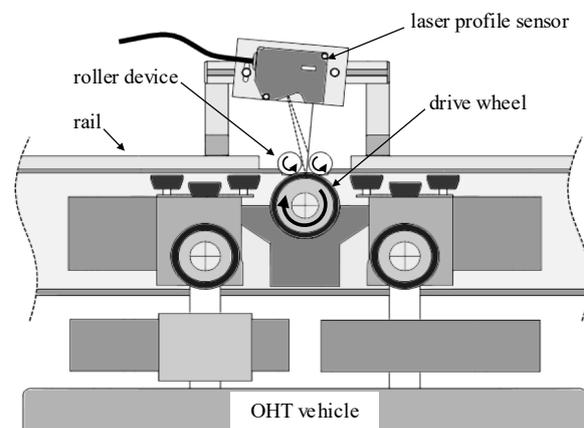
Figure 2. Section view of the inspection station and vehi
