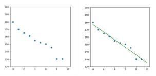
Figure 15. Schematic diagram of linear feature extraction for low-frequency signal
