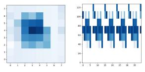
Figure 22. Raw data (left) and feature data (right) for moving behavior of CNC machine from IR sensor
