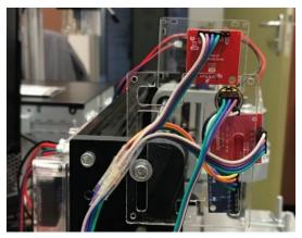
Figure 3. The first generation of hardware design, sensor stacking mode through DuPont line
