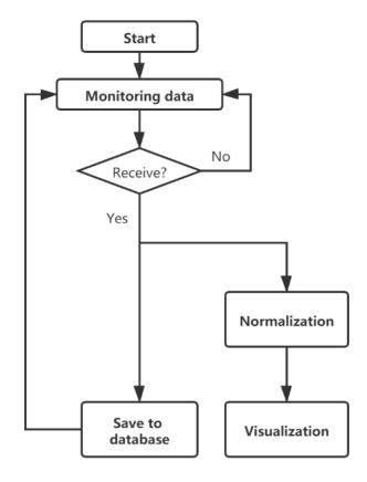
Figure 10. Flow chat of visualization program running on the application layer
