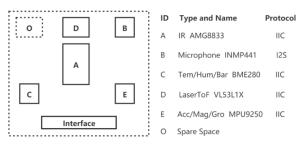
Figure 5. Schematic diagram and layout of our MSI sensor board
