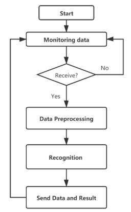
Figure 9. Flow chat of recognition program running on the processing layer
