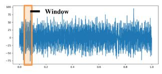
Figure 12. The raw microphone signal generated when the CNC machine rotates. The orange part is the Hamming window
