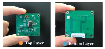
Figure 4. Top-Layer (Left) and Bottom-Layer (Right) of our modular scalable integrated sensor board
