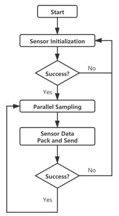
Figure 7. Flow chat of sampling program running on the physical layer
