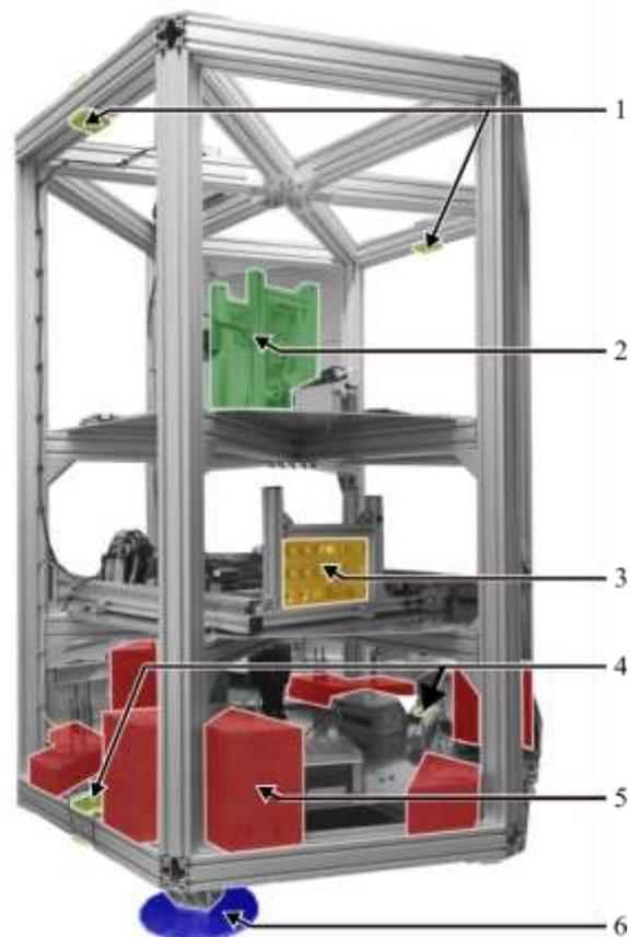
Figure 5. Experiment carrier including the experimental setup of MOONRISE, 1) upper centering rods with lifting points, 2) MOONRISE-setup, 3) control panel, 4) lower centering rods with integrated power connection, 5) ballast weights, 6) foot of the carrier
