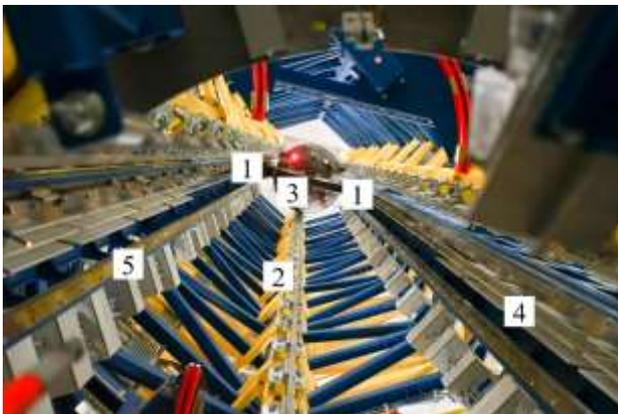
Figure 4. View from below, while gondola and experiment are in motion to the upper reversal point, 1) drive carts, 2) guide rails for gondola guidance, 3) traverse, 4) stators, 5) guide rails for drive guidance (based on source: LUH/Marie-Luise Kolb)
