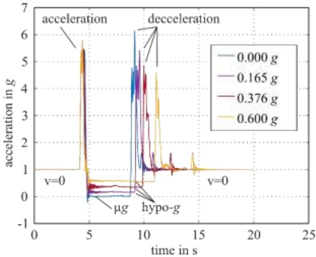
Figure 8. Acceleration curves of selected driving profiles
