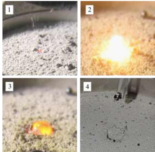
Figure 13. Melting of Moon regolith, 1) Melting process starts with some particles being ejected. 2) A sphere of molten simulant grows and 3) cools. 4) Sample after the process
