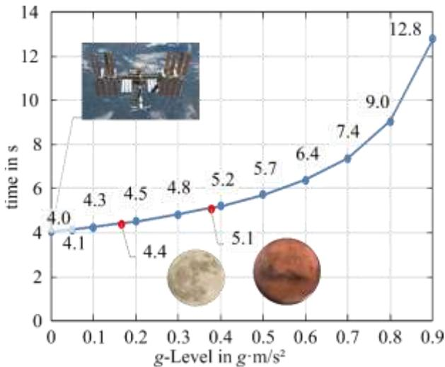
Figure 9. Duration in different simulated gravity conditions in the Einstein-Elevator
