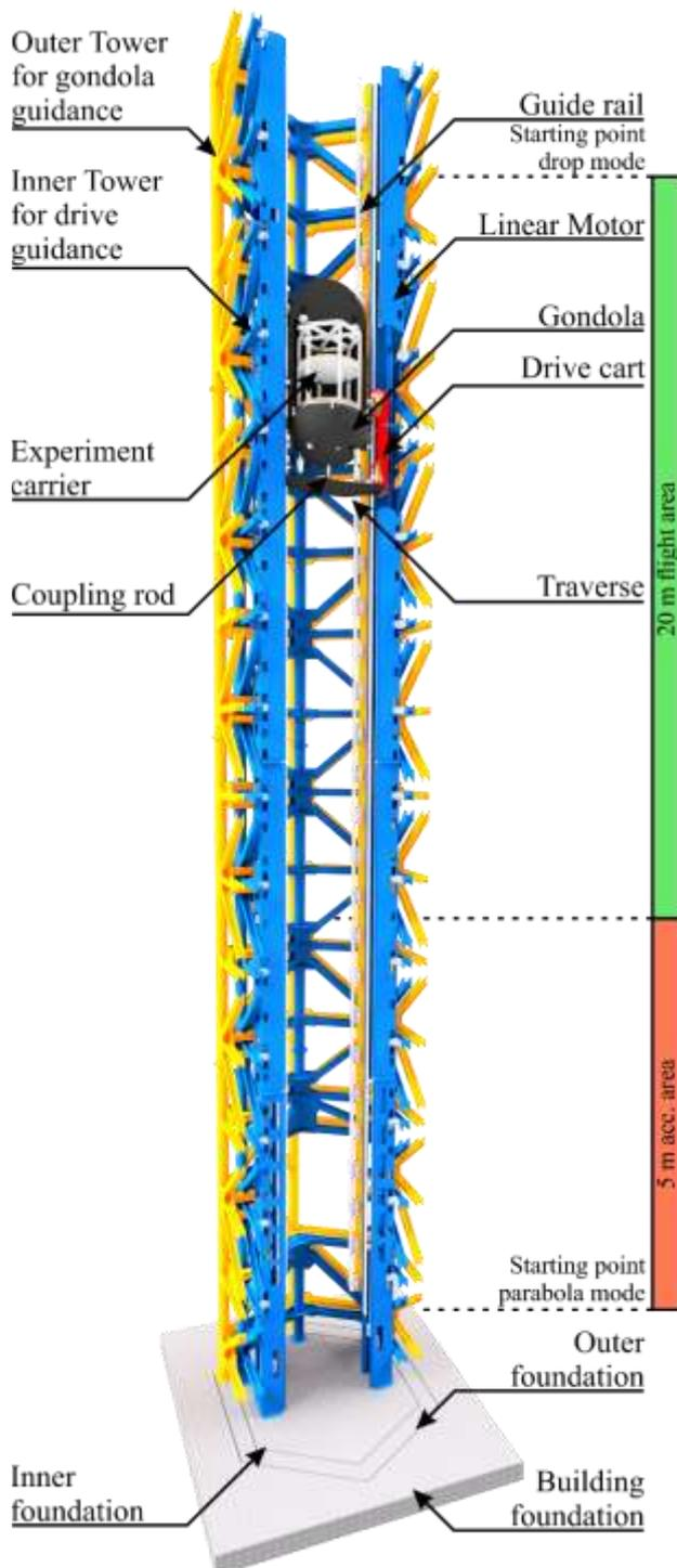
Figure 2. Design of the Einstein-Elevator
