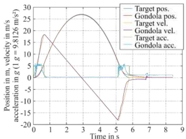
Figure 11. Position, velocity and acceleration of the gondola during flight (Moon-g: 2020-03-03UTC09-13-39)
