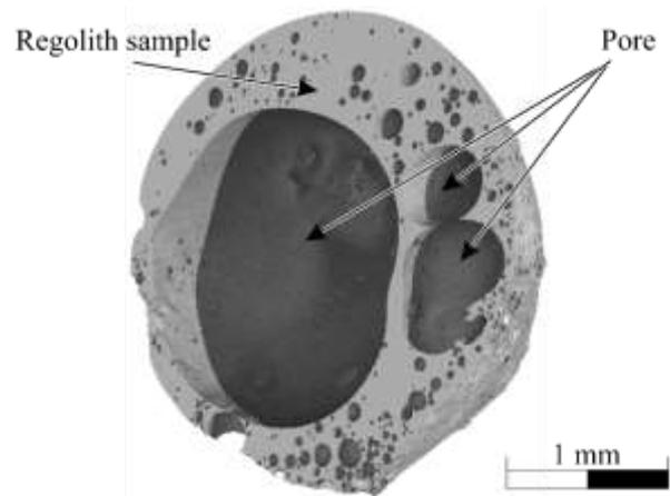
Figure 14. CT-scan of sample laser melted under lunar gravity
