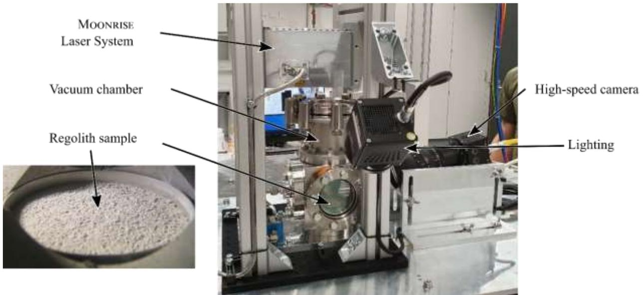
Figure 10. Experimental setup for laser melting of regolith under lunar conditions in the Einstein-Elevator
