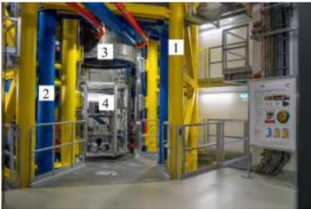
Figure 3. View inside the system at loading level, 1) outer supporting structure, 2) inner supporting structure, 3) gondola, 4) experiment carrier (based on source: LUH/Marie-Luise Kolb)
