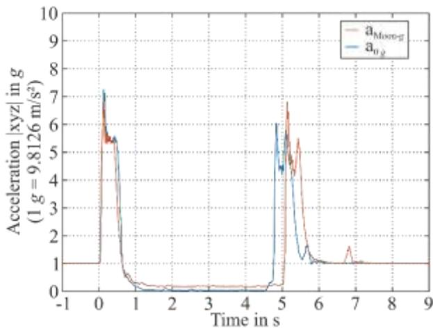
Figure 12. Acceleration [xyz] measured at Experiment Carrier during Flight (Moon-g: 2020-03-03UTC09-13-39, 0 g: 2020-03-10UTC08-58-01)
