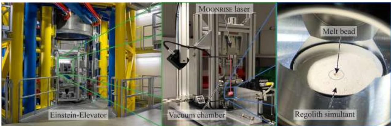
Figure 1. MOONRISE in the Einstein-Elevator, Left: Experimental setup inside the gondola (based on source: LUH/Marie-Luise Kolb). Middle: Flight hardware of the MOONRISE laser system. Right: Melt bead of regolith in the evacuated process chamber
