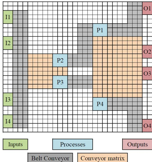
Figure 12. Layout: cost weight  $\alpha = 0.35$ , flexibility weight  $\beta = 0.65$ .
