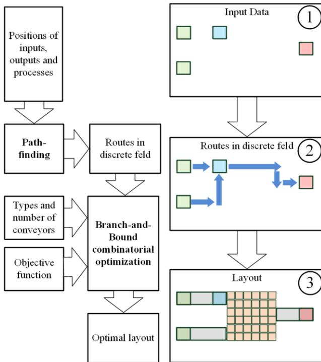
Figure 8. Sequence of the whole optimization process
