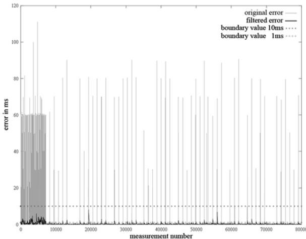
Figure 3. Synchronization accuracy with PTP-measurement in a busy network with and without filtering
