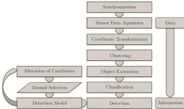
Figure 1. Toolchain for collaborative detection of autonomous transport vehicles
