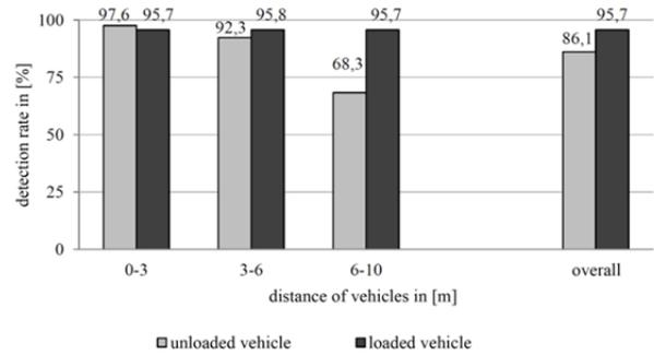
Figure 13. Diagram of the detection rate of extracted vehicle candidates with different loading
