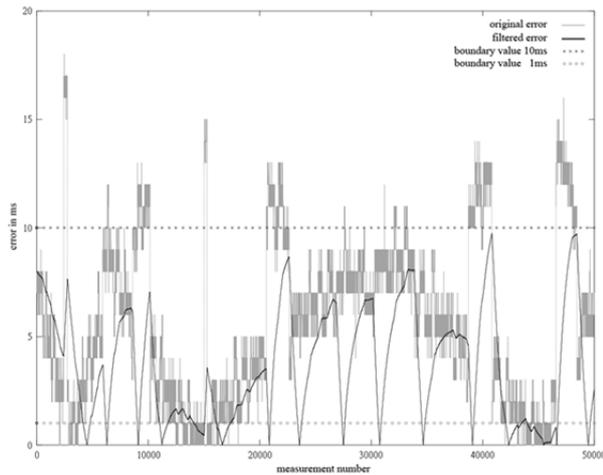
Figure 5. Synchronization accuracy with NTP-measurement in a busy network with and without filtering
