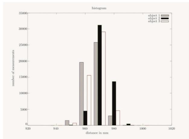
Figure 6. Histogram of distance measurements to different test objects with a distance of 1000 mm
