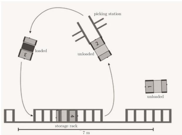
Figure 12. Logistical setup of the interconnected cellular transport vehicles
