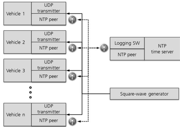
Figure 4. Setup for NTP-measurements
