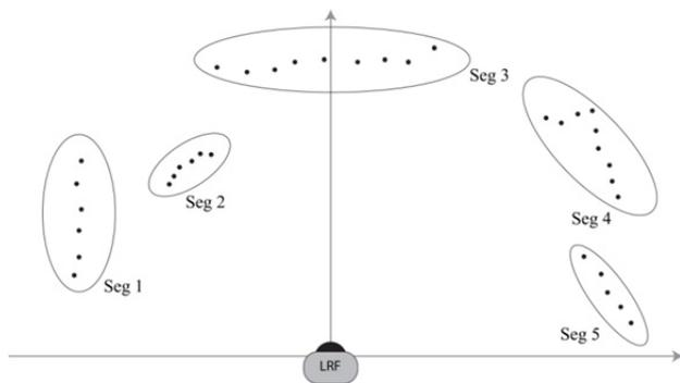
Figure 7. Clustering of a laser scanner point cloud
