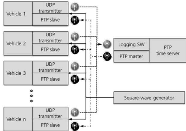
Figure 2. Setup for PTP series of measurements
