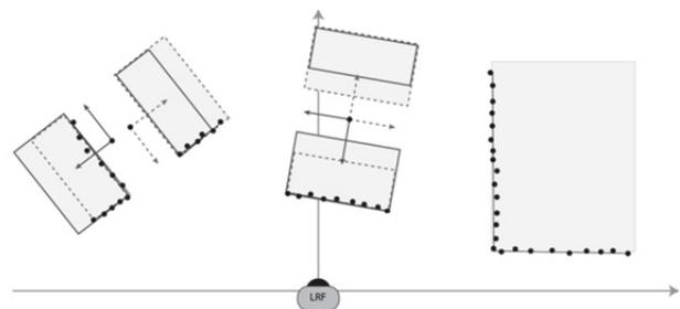
Figure 9. Recognition of geometrical forms; possible vehicle positions are highlighted gray
