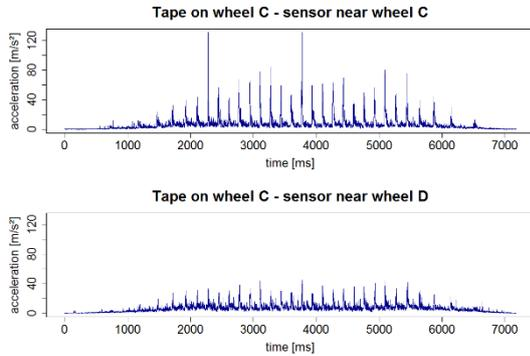
Figure 2.: Sensor Data tape on wheel a) wheel C b) wheel D
