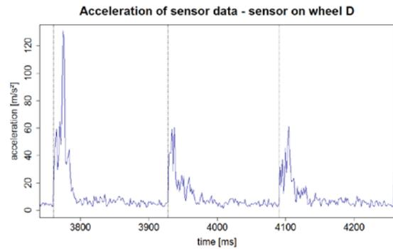
Figure 5.: Acceleration of the sensor data over 3 wheel rotations Sensor on the wheel D
