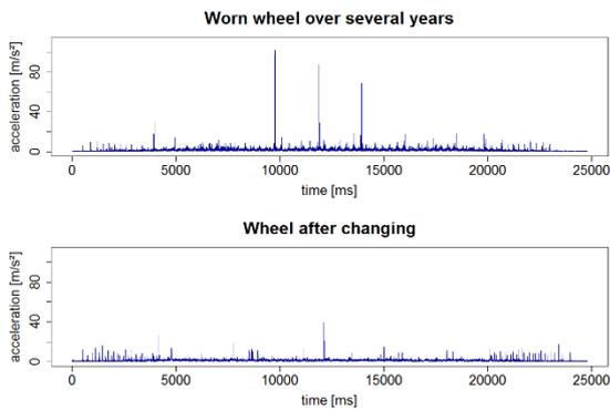
Figure 8.: Homing ASRS a) before maintenance b) after maintenance
