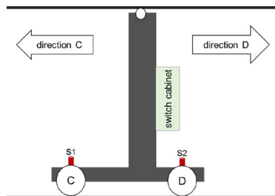
Figure 1.: Schematic structure of an ASRS and placement of the sensors
