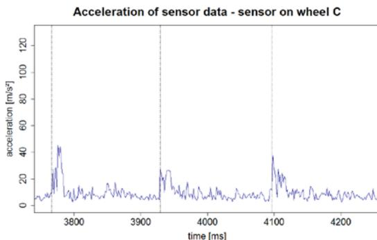
Figure 4.: Acceleration of sensor data over 3 wheel rotations Sensor on wheel C
