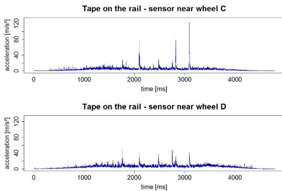
Figure 6.: Sensor data tape on rail a) Wheel C b) Wheel D
