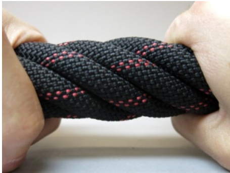
Figure 2. Hand model showing closing twist “ +\omega ”
