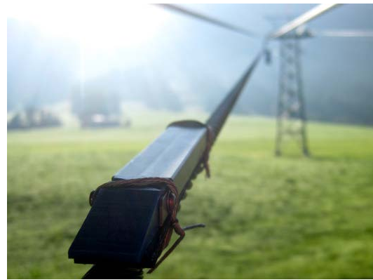
Figure 7. Digital rotation measurement at a jigback aerial tramway
