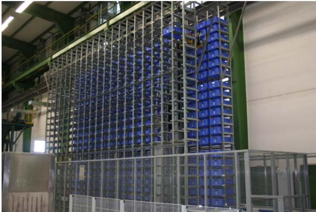
Figure 3. The Automatic Small Parts Warehouse at the Institute of Logistics and Material Handling Systems at the Otto-von-Guericke University Magdeburg
