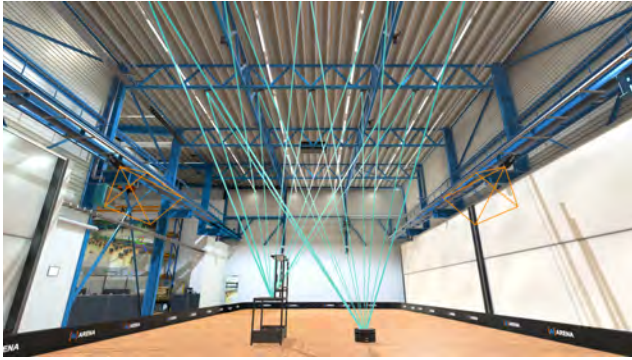
Figure 1: Rendering of our research facility, depicting the camera system used for our recordings. Enlarged representations of two RGB cameras are shown in orange. Reflected rays captured via the motion capture system are shown in cyan.
