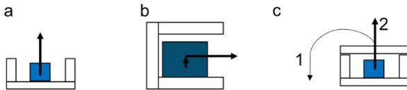
Figure 1: A set of pick-and-place tasks in material handling that were investigated with different start positions to find similarities in the movements for a) picking an object from a box, b) removing an object from a shelf and c) first opening a box then retrieving the content.
