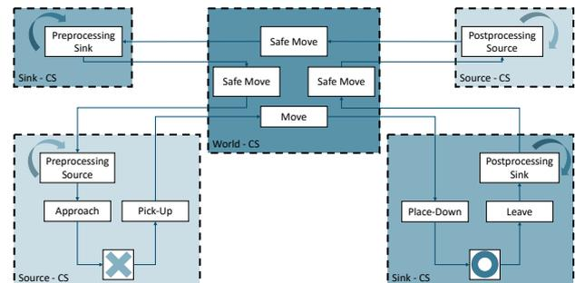
Figure 5.: Conceptual description of the 5+5 Steps of the Material Handling Loop with trajectory segments (white boxes), the grasp (x) and the release (o) point and the reference coordinate systems (CS) source, sink and world, relative to whom the trajectories are executed.
