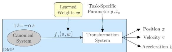
Figure 3: Summary of the one-dimensional DMPs with a canonical system, which specifies the non-linear part and thus can react to new task parameters [8].
