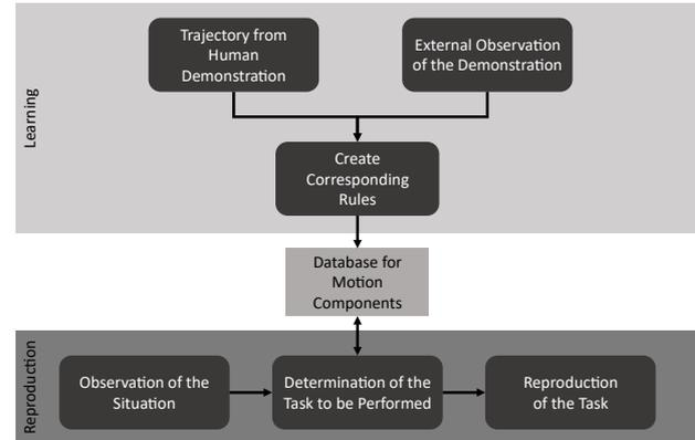
Figure 6.: Sequence of the two-stage process of learning and reproduction with the exchange of the acquired rules via a database that can be accessed from both subprocesses.
