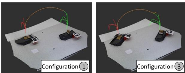
Figure 11.: Visualization of the adapted trajectories from the demonstrated configuration (left) to the 45° rotated configuration (right) with  $\Pi_{pick}$  in red,  $\Pi_{move}$  in orange and  $\Pi_{place}$  in green.
