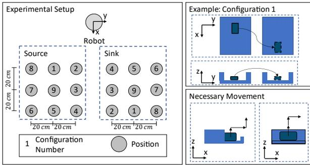
Figure 10.: Setup for the second experimental series to compare the presented approach with unsegmented DMPs performing the described task with start position in source and goal position in sink for each configuration number.
