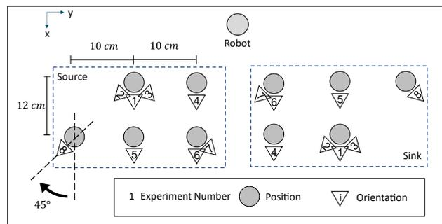
Figure 9.: Experimental setup for evaluating the adaptability of the approach by spreading source and sink positions and rotating them.
