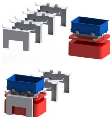
Figure 2: Dedicated stations for the autonomous loading and unloading process of the material units (KARIS PRO concept)
