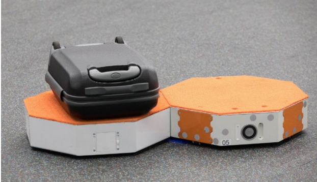
Figure 11.: Implementation of buffer function on a carrier (© Thomas Willemsen – Fraunhofer IML)
