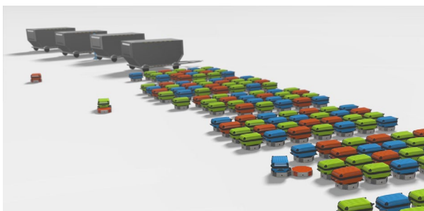
Figure 3.: Buffering of baggage for ULD-specific consolidation on apron
