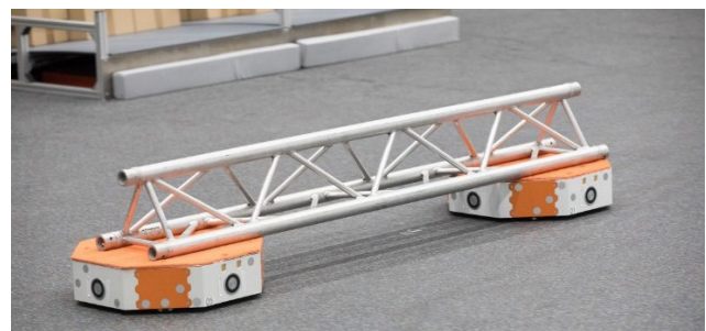
Figure 10.: Collaborative transport of a crossbeam (© Michael Neuhaus / Fraunhofer IML)
