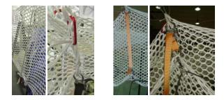
Figure 6: Shortener – advancement of Isilink® with highstrength filaments for 3d transmission of force (l.), clamping lock straps (r.)
