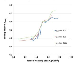
Figure 5: Sliding behavior of anti-skit system after different resting times
