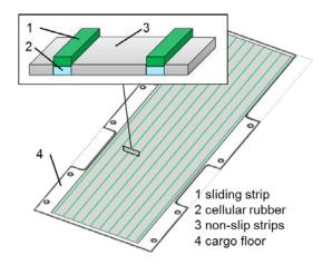
Figure 4: Structural composition of anti-skit system
