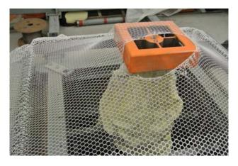
Figure 2: Determination of the main breaking force [STFI e.V.]
