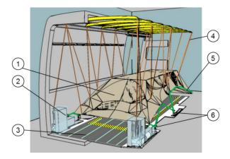
Figure 1: Automatic load securing system in lashed position
