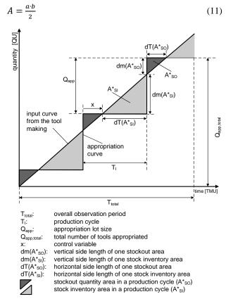
Figure 4: Geometrical relationships in the throughput diagram of the tool issuing store
