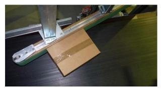
Figure 7. Orientation via belt deflector (topview)
