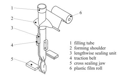
Fig. 2: Vertical Form Fill Seal Machine [DIN00]
