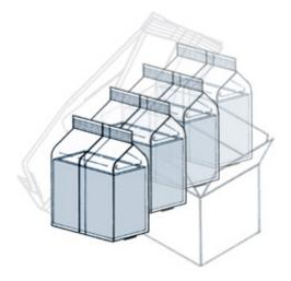
Fig. 4: Standing block bottom bags [rov05]
