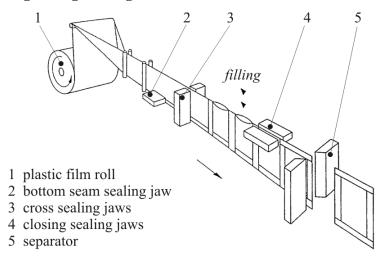
Fig. 1: Horizontal Form Fill Seal Machine [DIN00]
