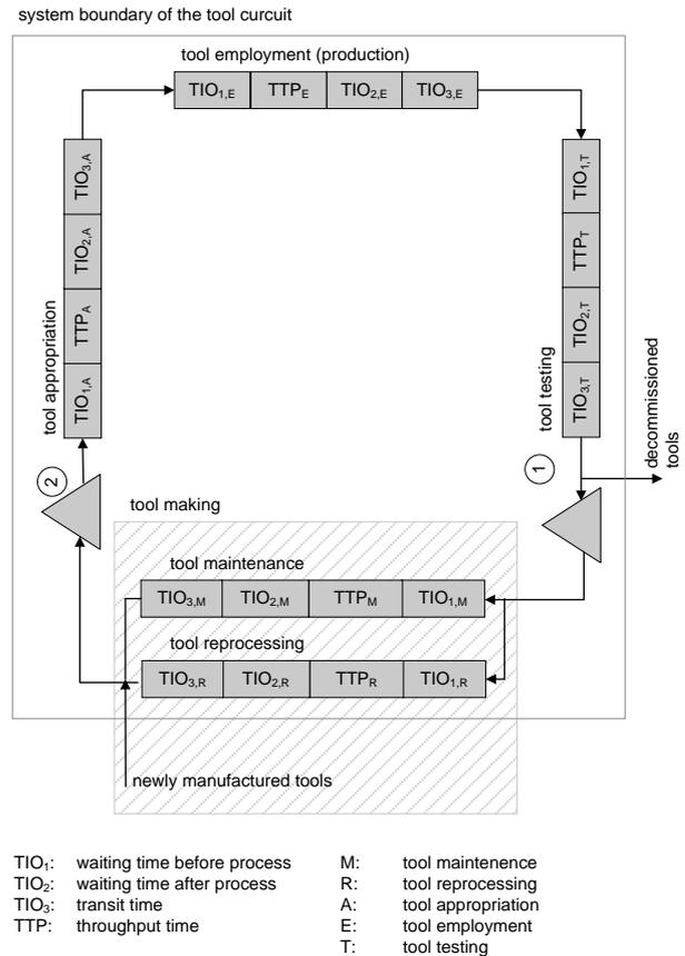
Figure 1: Modeled tool circuit
