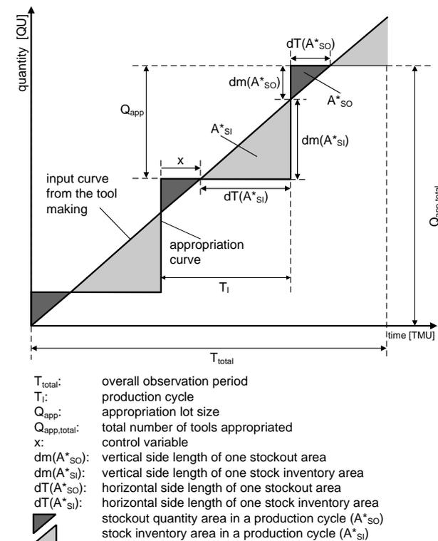
Figure 4: Geometrical relationships in the throughput diagram of the tool issuing store
