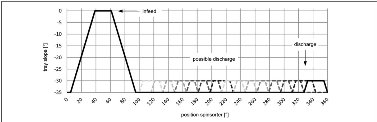
Figure 3. Tray slope during one rotary sorter cycle
