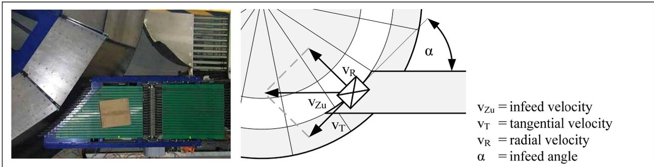
Figure 8. Infeed angle and infeed velocity, according to [Hir03]
