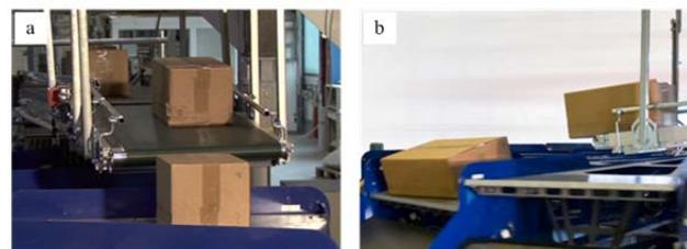
Figure 10. Overhead infeed, a) front view, b) side view
