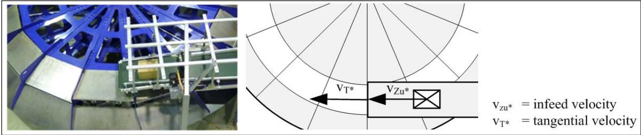
Figure 11. Overhead infeed and infeed velocity
