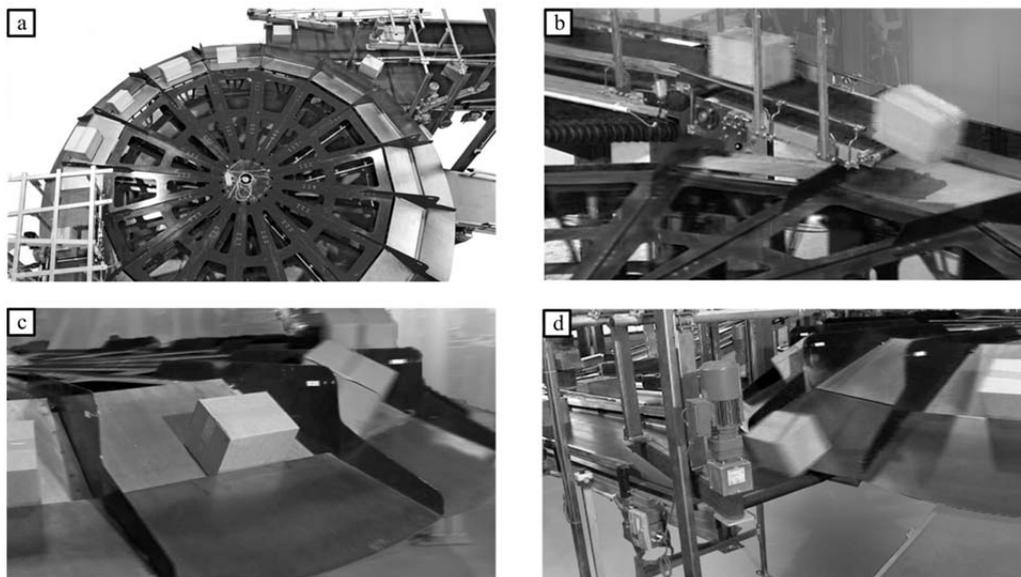
Figure 4. Sorting with rotary sorter (a – construction; b – infeed; c – conveying; d – discharge)
