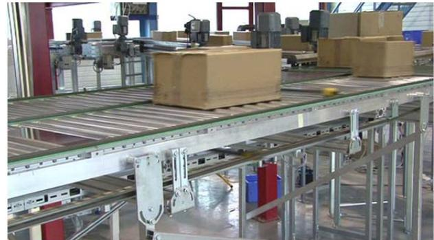
Figure 6. Synchronization conveyor (positioner), by Tansnorm System
