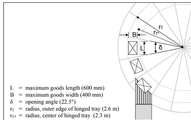
Figure 2. Geometrical relations of prototype (topview)
