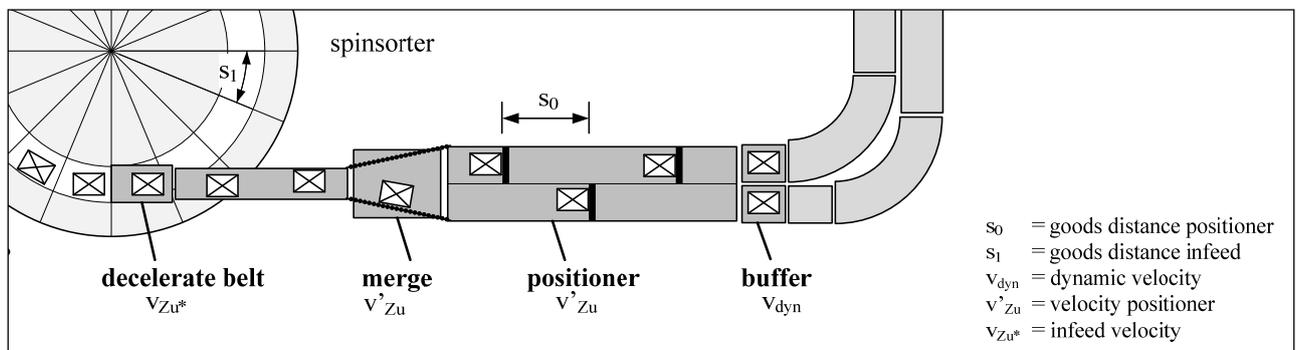
Figure 12. Schematic infeed line with overhead infeed
