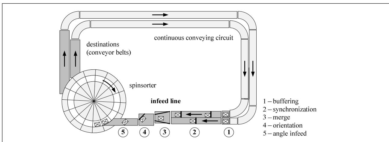
Figure 5. Rotary sorter with continuous conveying circuit and newly designed infeed line
