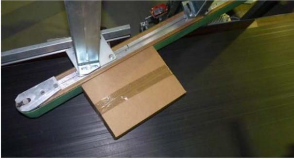
Figure 7. Orientation via belt deflector (topview)
