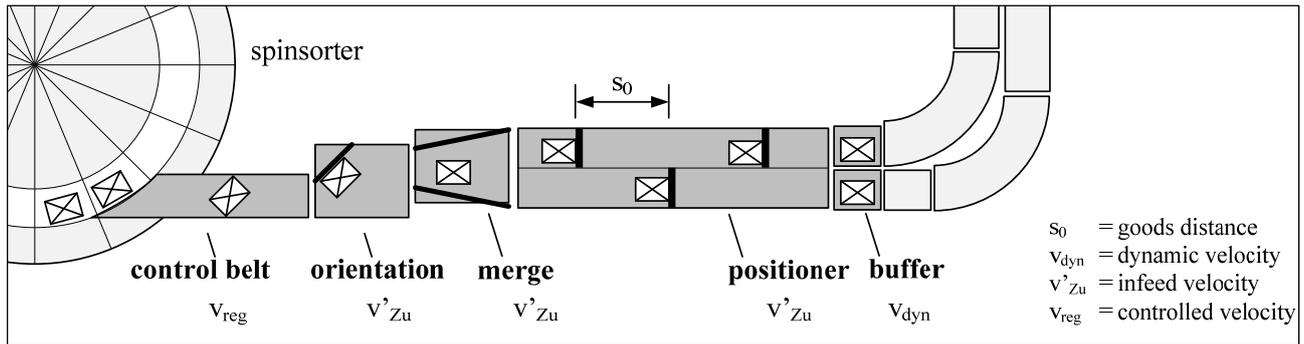
Figure 9. Schematic infeed line with angle infeed
