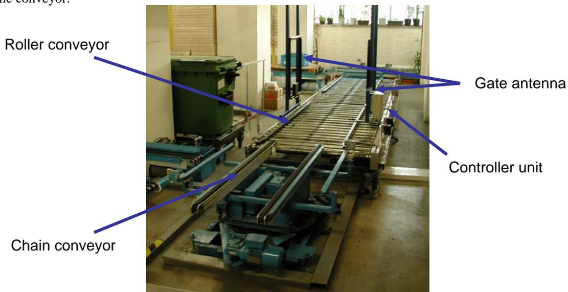
Fig. 1: Test installation at IFT
