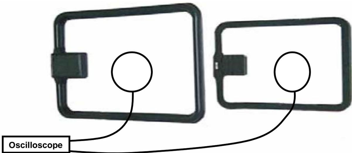
Fig. 4: Basic and supplementary antenna with principal measurement scheme for signal adaptation
