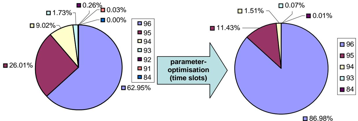
Fig. 16: Increase of recognition rate due to parameter optimisation in preliminary test setup with KLTs and 96 transponders (example)
