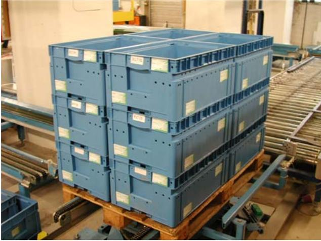
Fig. 7: KLT setup with 96 transponders (eight for each KLT)
