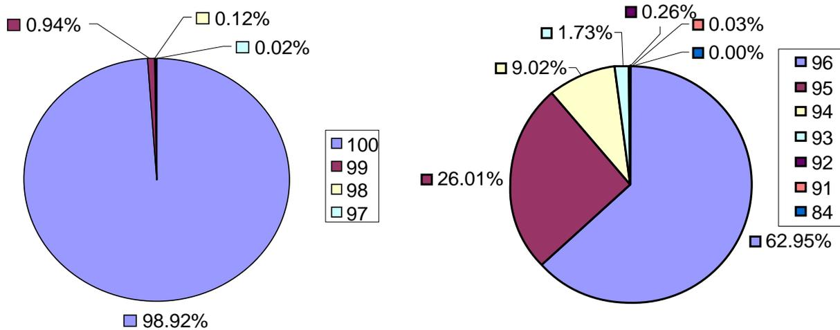
Fig. 13: Recognition rate in a two-dimensional plate setup (100 transponders, left) versus a three-dimensional KLT setup (96 transponders, right) with identical parameter settings (example)
