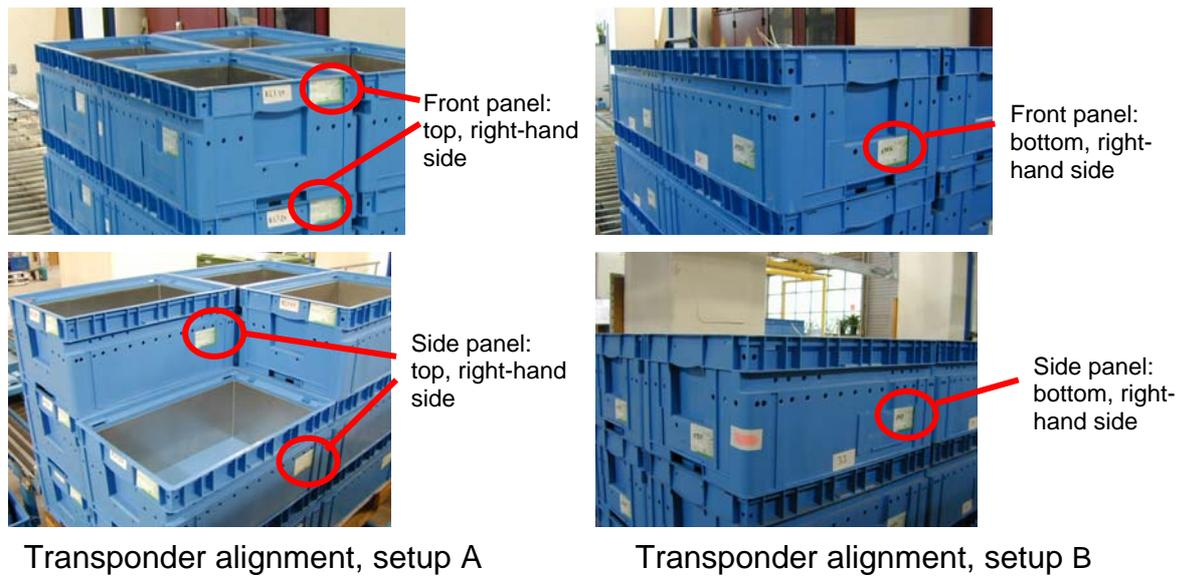
Fig. 2: Transponder position in setup A and B in comparison
