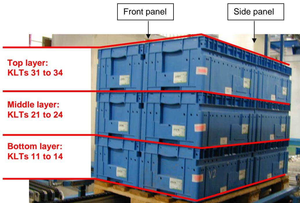
Fig. 9: Stacked KLT layers on pallet and numbering of containers
