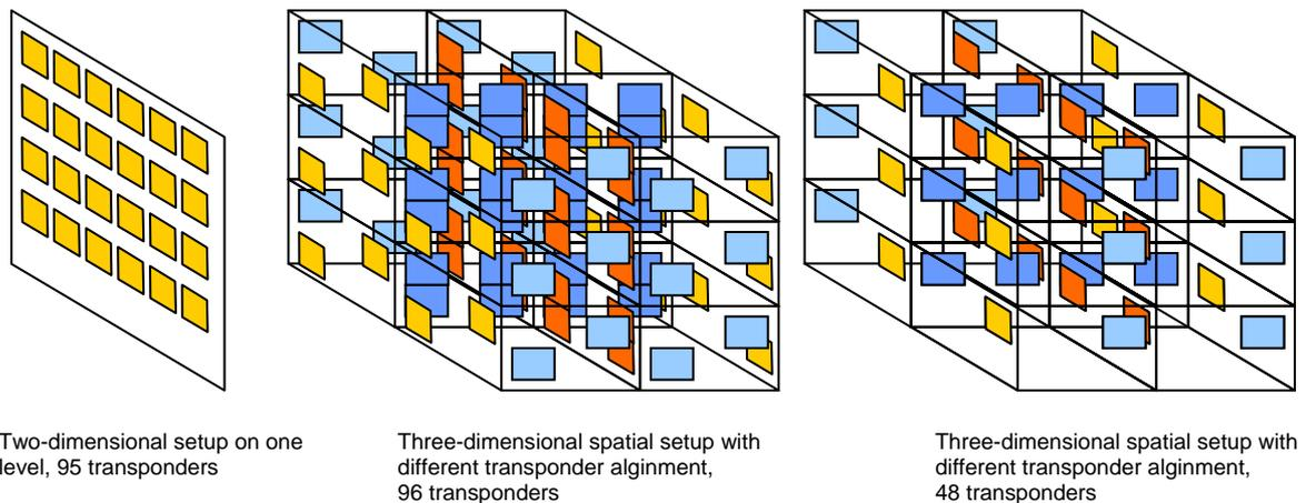
Fig. 14: Spatial transponder alignment for the plate tests and the KLT setups with 96 and 48 transponders
