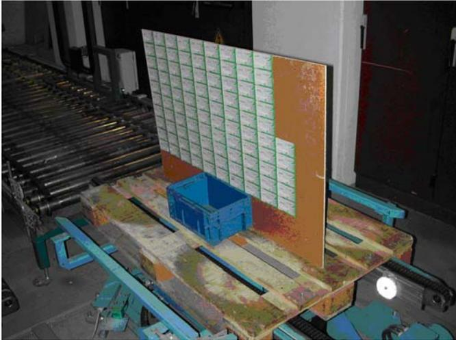
Fig. 6: Two-dimensional preliminary test setup with 95 transponders
