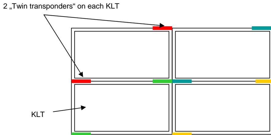
Fig. 11: KLTs with two transponders each (bird view)
