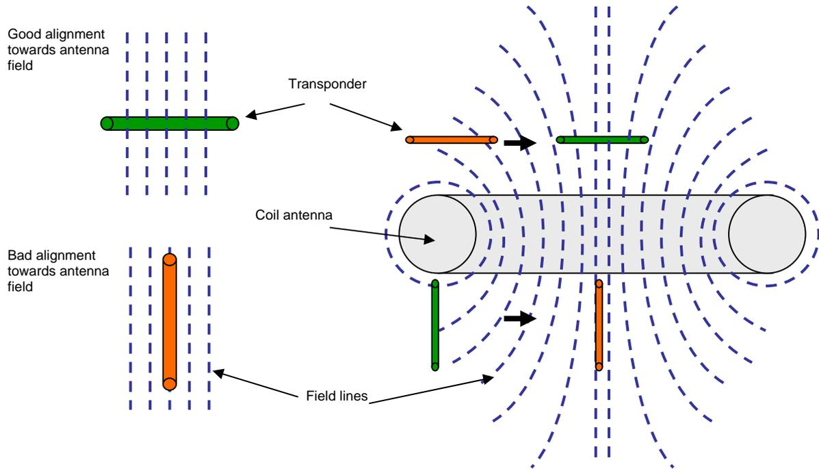
Fig. 15: Transponder alignment with respect to the field lines and within the antenna field
