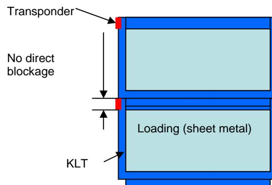
Fig. 12: Mounting the transponders outside of the usable loading level
