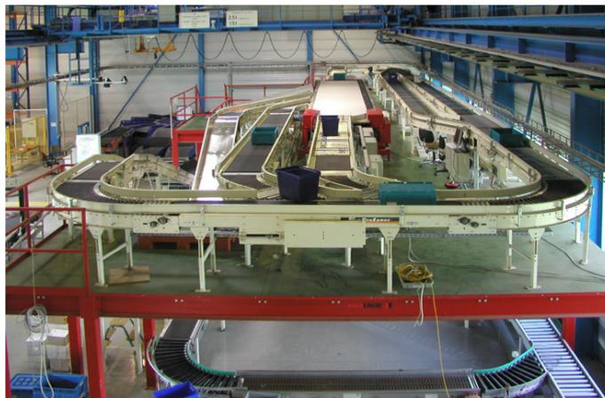
Fig. 1 Conveyor and sorter equipment
