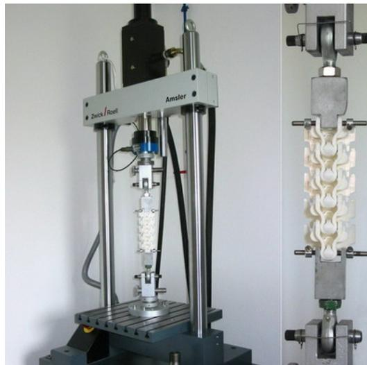
Fig. 1: Dynamic testing machine and fixation of the tested chains
